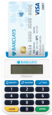
A PINsentry is a security device that generates single-use codes when used with your authentication card or Barclays debit card.
